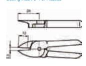
BK1030-07 Carbide cutting insert 0° for steel
