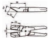
BK1065-07 Carbide cutting insert 0° for steel
