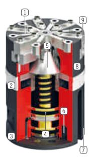
1 Ejector jaw - to shift off the O-ring 2 Stroke adjustment - for adjustment of the spread stroke 3 Energy supply - possible from several sides (4) Drive - two single-acting pneumatic cylinders 5 Force transfer - direct via taper 6 Mounting and positioning - axial, on the gripper bottom 7 Sensing slot - mounting and positioning of magnetic field sensors 8 Robust, lightweight housing - Hard-coated aluminum alloy 9 Gripper jaw - individual gripper finger mounting
